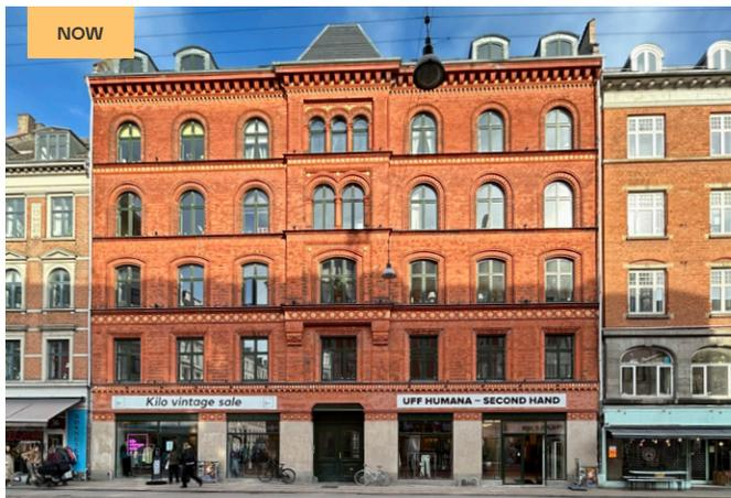
We removed old signs and attached panels from the storefront and renovated one half of it. Unfortunately, we were unable to find any of the original facade under the other half, so we rebuilt it from scratch using handmade stones. Finally, new window sections were installed throughout the storefront. The work was carried out by skilled and proud craftsmen who meticulously cleaned, reused, and rebuilt – all with great respect for the property's character and qualities.
